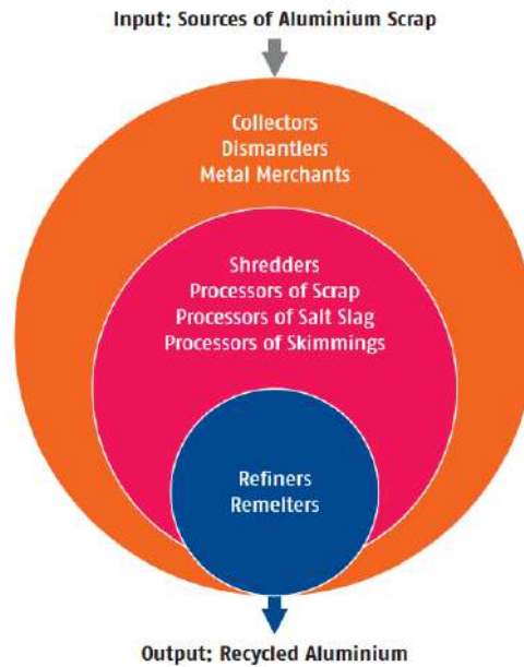
Figure 2. Structure of the Aluminium Recycling Industry [world-aluminium.org (alu.org)]
