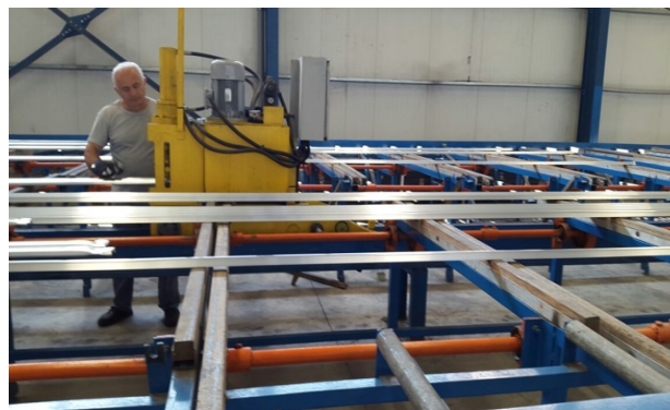
Figure 5. Tensile process of the AA6063 profiles
